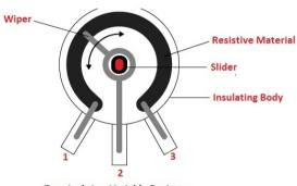
Terminals in a Variable Resistor
